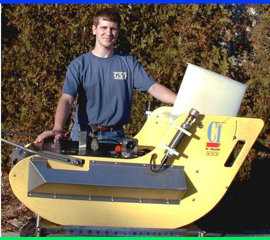
An undulating oceanographic recorder, towed behind a ship, is used to collect ecological parameters needed to assess the state of the marine ecosystem.
